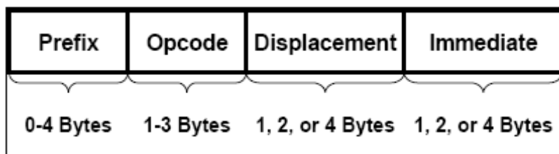
Figure 4.23: Simplified IA-32 Instruction Format.
